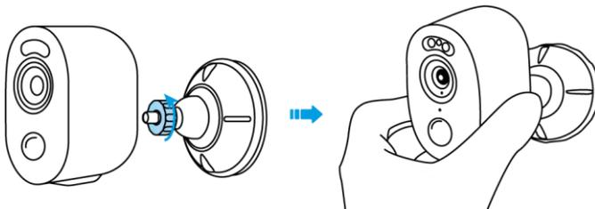
**Step 4.** Secure the camera by turning the part on the mount identified in the chart clockwise.
