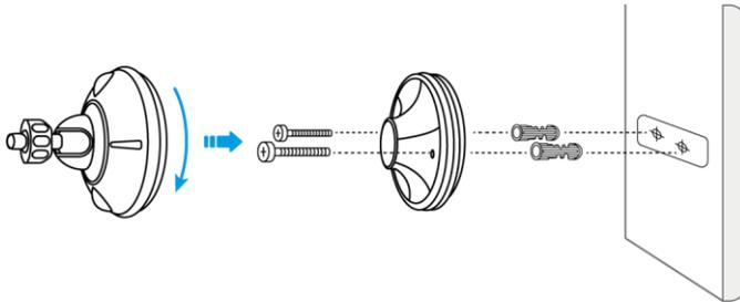
**Step 3.** Screw the camera to the mount. Adjust the camera's angle to get the best field of view.
