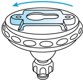
**Step 2.** Drill holes with the mounting template and screw the base of the mount onto the wall. Then attach the other part of the mount to the base.
